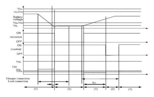
Notes: (1) Normal condition (2) Overcharge voltage condition (3) Overdischarge voltage condition (4) Overcurrent condition
